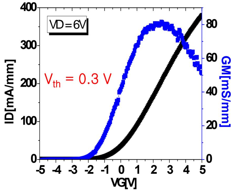
(1) Channel thickness of 400 nm
