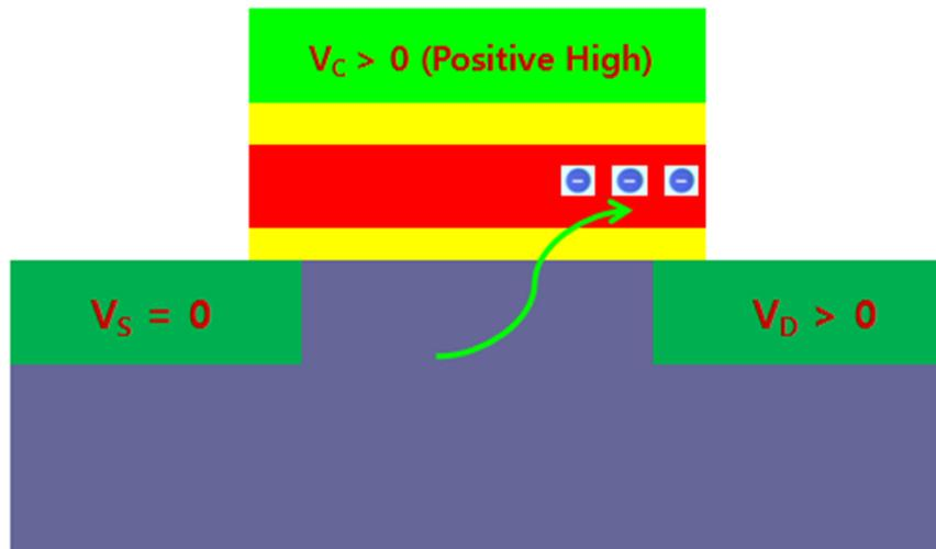
✓ The CHE mechanism, where electrons gain enough energy to pass the oxide-silicon energy barrier, thanks to the electric field in the transistor channel between source and drain.
