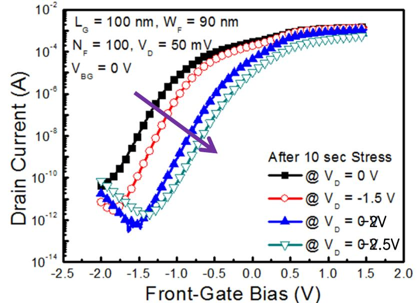
➤ High drain biasing can lead to charge trapping in the  $\text{Si}_3\text{N}_4$  buried layer.
