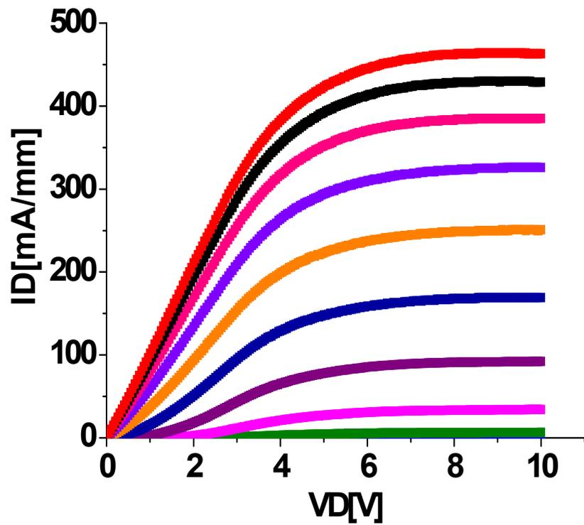
(1) Channel thickness of 400 nm
