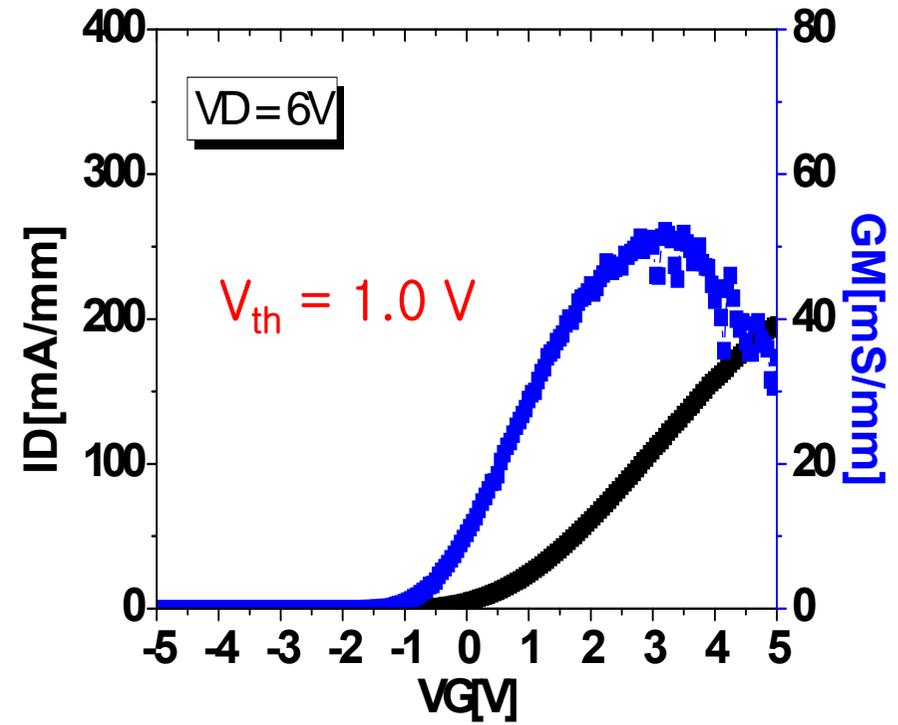
(2) Channel thickness of 250 nm
