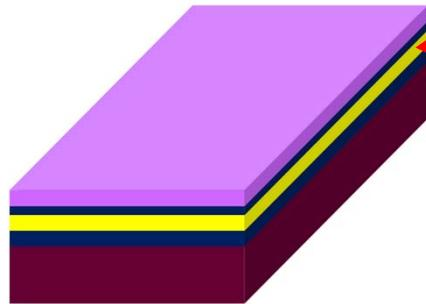
← **Oxide/Nitride/Oxide Structure**
