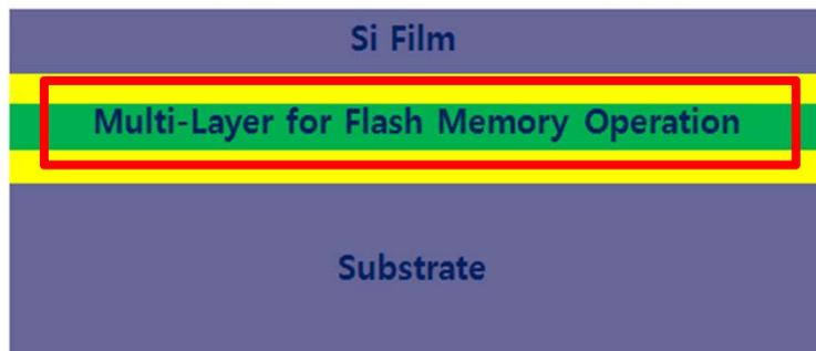
Oxide/Nitride/Oxide Multi Layer
